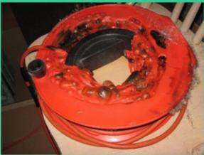
Use the **appropriate length** extension cord. **Never** use an extension cord while it is coiled or looped. It can overheat quickly.
