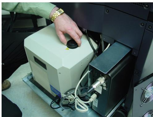
Figure 10.4 Removing the fill cap
