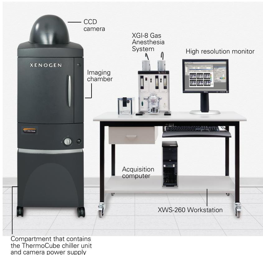
**Figure 1.1** IVIS® Spectrum Imaging System
