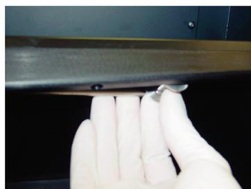
The stage lock down bar is located at the bottom front edge of the imaging platform.
